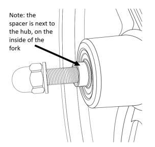
The Right side of the wheel will use the wider 8.5mm spacer between the hub and fork as shown below.
