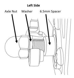
Then use a 16mm wrench to tighten the axle nuts firmly. As shown below.
