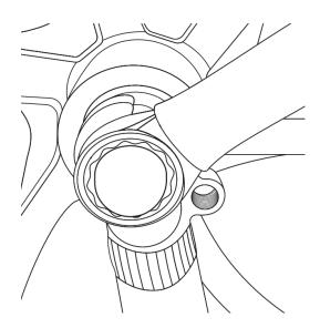
Flip the bike over onto the wheels and be sure to check that the handlebars are aligned with the front tire. Then tighten both sides of the stem to the fork using a 4mm Allen wrench, tighten to 45 IN-LBS or 5 Nm.
