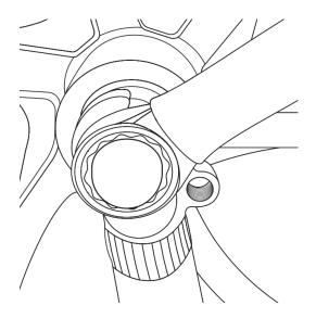
Attach the pedals to the bike by using a 15mm wrench, be sure to identify the correct pedal for the correct side, there is an R or L marked on the end of the pedal bolt. Be sure to note that the left pedal is reverse threaded. It is recommended to add general purpose grease to the threads before installing the pedals. (Right and Left is determined when sitting on the bike)
