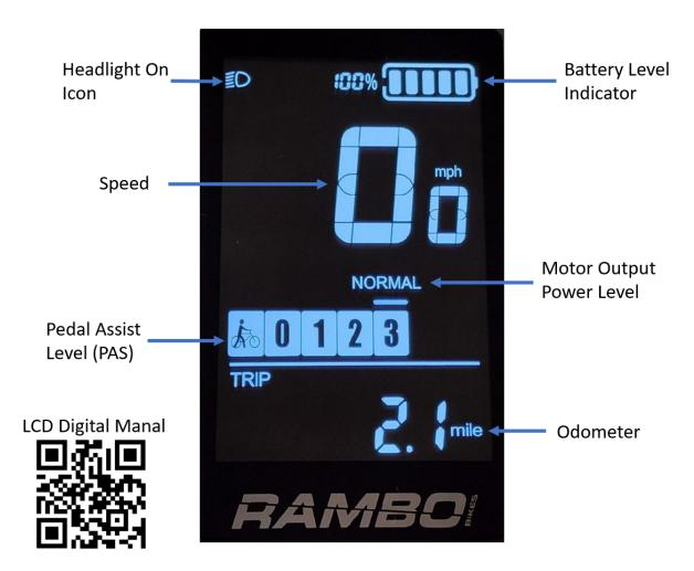
Each PAS (Pedal Assist Level) is approximately 20% motor power. Level 1 is 20%, Level 2 is 40%, Level 3 is 60%, Level 4 is 80% and Level 5 is 100% motor power.
