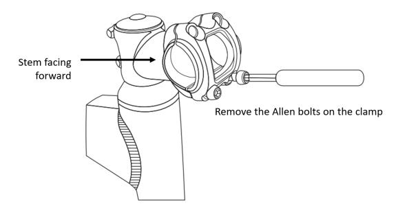
Next, install the handlebars to the stem using a 4mm Allen wrench. Be sure to tighten the Allen bolts in a cross pattern when tightening. Tighten to 45 IN-LBS or 5 NM (Make sure the stem is pointed forward) as shown below.
