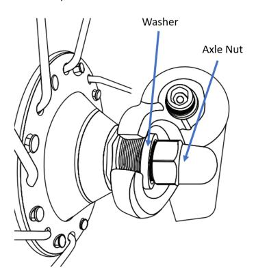
Then use a 15mm wrench to tighten the axle nuts firmly. As shown below.
