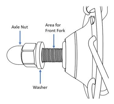
You can also remove the axle nut and washer then reinstall once the wheel is on the front fork.
