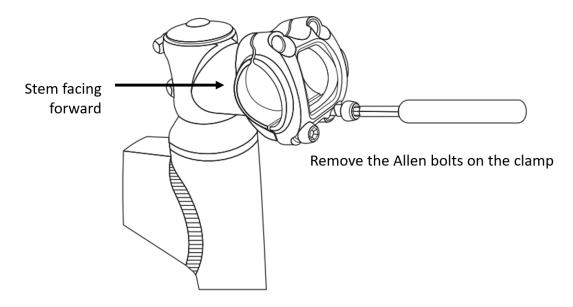
Next, install the handlebars to the stem using a 4mm Allen wrench. Be sure to tighten the Allen bolts in a cross pattern when tightening. Tighten to 45 IN-LBS or 5 NM (Make sure the stem is pointed forward) as shown below.
